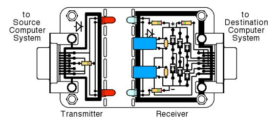
The transmitter converts electrical signals from the source computer system to optical form, using a pair of red LEDs. The receiver uses a pair of phototransistors to convert the optical data back to electrical form. The top LED/phototransistor pair transmits positive signals, while the bottom pair transmits negative signals.
