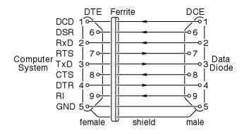
**Note:** All diagrams of cable connectors given here show the pinout as it appears when looking at the face of the connector from the outside.
