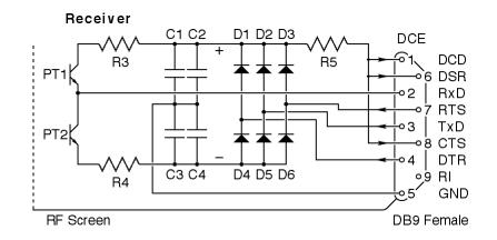
PT1 and PT2 – NPN phototransistors; PNA1801LS, able to handle a maximum forward current of 20 milliamps and a forward voltage of 15 volts or more, with a collector current of at least 3mA at 500 Lux, peak sensitivity near 800nm, and a 4 $\mu$ s response time. Redesign with a transistor amplifier on each phototransistor should increase the data rate.
