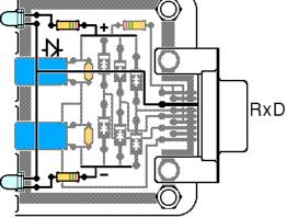
**The shielding loop** operates identically to that in the transmitter, except that it is also in electrical contact with the screws attaching the RS-232 Data Diode to its case.
