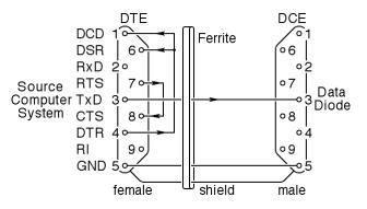
8), and the DTR output (pin 4) is fed back into the DSR and DCD inputs (pins 1 and 6). These connections are identical to those established by a standard "loopback connector" used for serial port testing. A ferrite bead should be used at the computer end.
