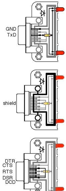
In the alternative cable suggested for connecting the source computer system to the RS-232 Data Diode, these "loopback" connections are wired inside the cable.
