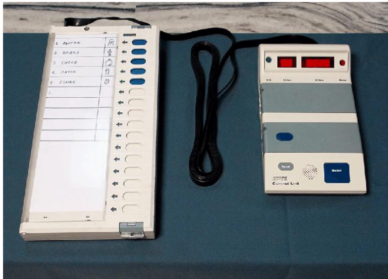
Figure 1.1, An Indian EVM, made up of a balloting unit (left) and control unit (right). [7]
